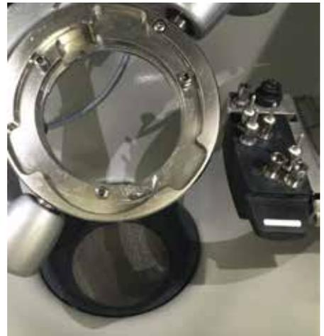
Corresponding to the former sieve No 1 for wet processing. This sieve should no longer be used. The new sieve No 1 was supplied to dealer for all inLab MC X5 machines (serial number < 40158). If necessary please contact your dealer.
